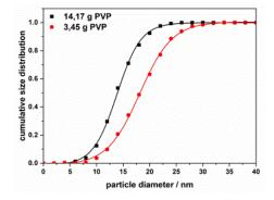
Figure 1. Cobalt particle size as a function of the different amount of PVP.
