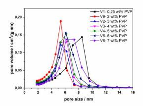
Figure 2. Pore size distribution as a function of the different amount of PVP
